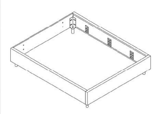
attach the metal profiles shown as in the picture that carry the wooden cover
